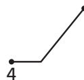
Graph 4 shows the cyclist not moving for the first part of the time interval and then riding at a steady rate for the rest.
