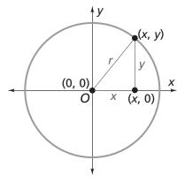
Applying the Pythagorean Theorem to the right triangle, you have  $x^2 + y^2 = r^2$ . This equation would be true for any point (*x*, *y*) on the circle. So, the equation represents the relationship for all points on the circle.
